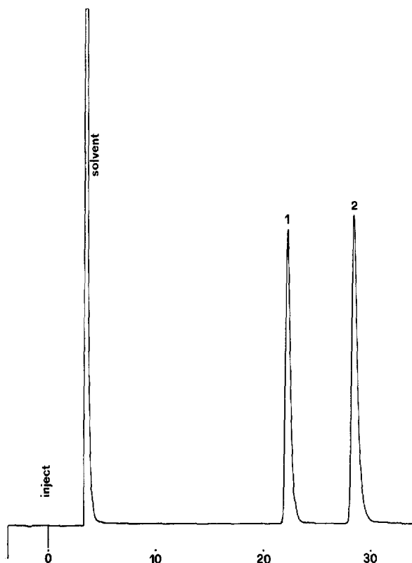
Fig. 1. HPLC separation of khellin and visnagin standards. 1 = Khellin; 2 = visnagin. Ordinate: absorbance (254 nm); abscissa: retention time (min). Operating conditions as described under Experimental.
